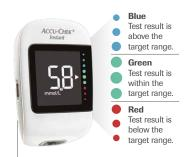
Press to eject test strip A strip ejector for quick, hygienic removal. \*The target range is set by default at 3.9–8.9 mmol/L. To change the target range, pair the meter to a mobile device, or connect it to a PC with diabetes management software installed.
