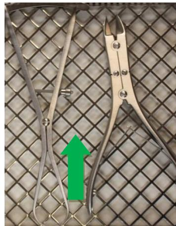
Preliminary rinsing (cold, if applicable fully demineralized water without additives) is followed by chemical. The chemical cleaning should take place at **40°C -60°C** for at **least 5 minutes**.
