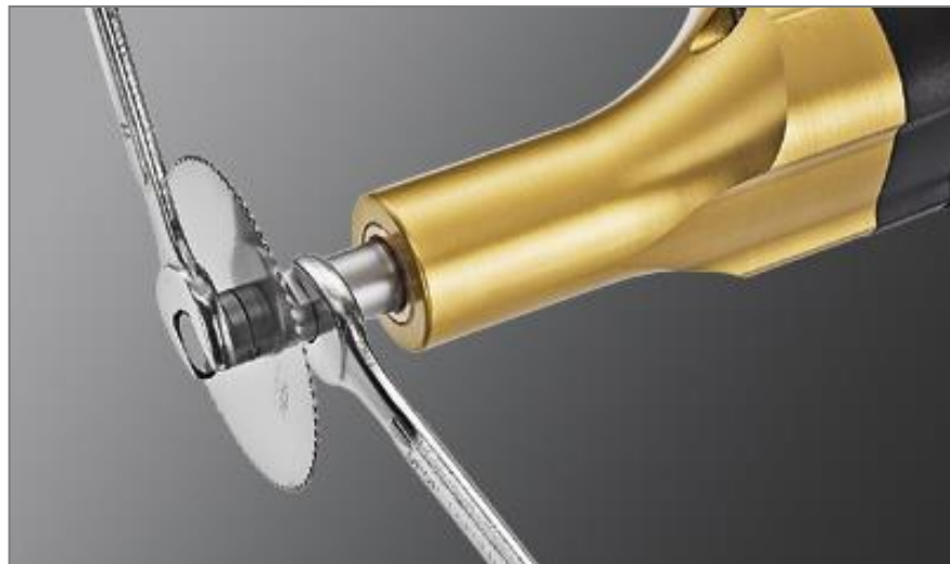
Fig. 1: Releasing the retaining screw
